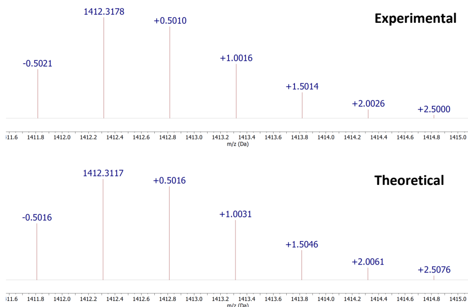
Figure S2c-2. Isotope distributions of ion \text{H8}\cdot\text{OV}^{2+} in the 1:2 mixture of \text{H8} and \text{OV}^{2+}\cdot(\text{PF}_6^-)_2 (upper: from ESI-QTOF spectrum; bottom: from computer simulation). The mass difference between isotope peaks is about 0.5 (1/2).
