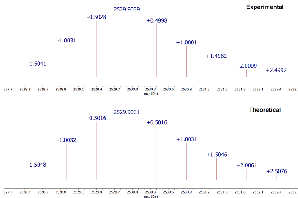
Figure S3b-4. Isotope distributions of ion \text{H16}\cdot\text{OV}^{2+} in the 1:2 mixture of H16 and \text{OV}^{2+}\cdot(\text{PF}_6^-)_2 (upper: from ESI-QTOF spectrum; bottom: from computer simulation). The mass difference between isotope peaks is about 0.5 (1/2).
