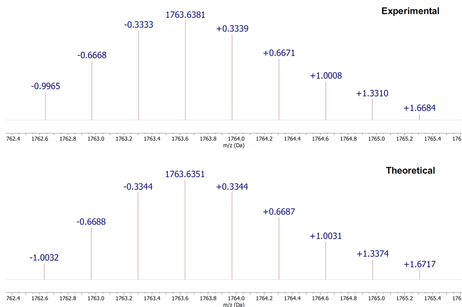
Figure S2a-3. Isotope distributions of ion (\text{H8})_2\cdot\text{OV}^{2+}\cdot\text{Na}^+ in the 2:1 mixture of H8 and \text{OV}^{2+}\cdot(\text{PF}_6^-)_2 (upper: from ESI-QTOF spectrum; bottom: from computer simulation). The mass difference between isotope peaks is about 0.33 (1/3).
