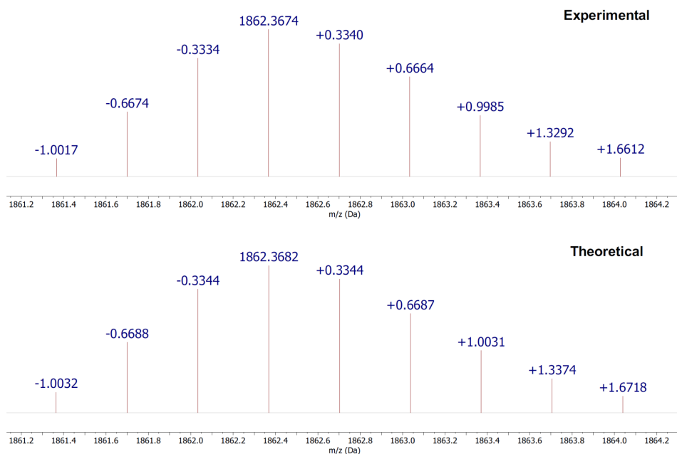
Figure S3b-3. Isotope distributions of ion \text{H16}\cdot(\text{OV}^{2+})_2\cdot\text{PF}_6^- in the 1:2 mixture of H16 and \text{OV}^{2+}\cdot(\text{PF}_6^-)_2 (upper: from ESI-QTOF spectrum; bottom: from computer simulation). The mass difference between isotope peaks is about 0.33 (1/3).
