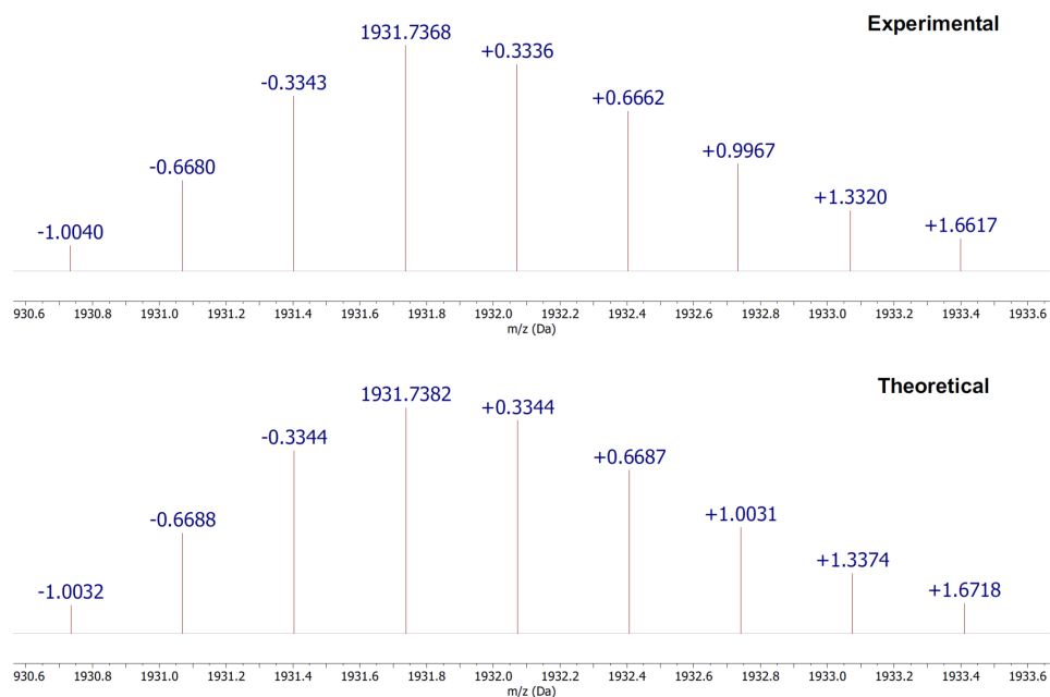
Figure S2b-3. Isotope distributions of ion (\text{H8})_2 \cdot (\text{OV}^{2+})_2 \cdot \text{PF}_6^- in the 1:1 mixture of H8 and \text{OV}^{2+} \cdot (\text{PF}_6)_2 (upper: from ESI-QTOF spectrum; bottom: from computer simulation). The mass difference between isotope peaks is about 0.33 (1/3).
