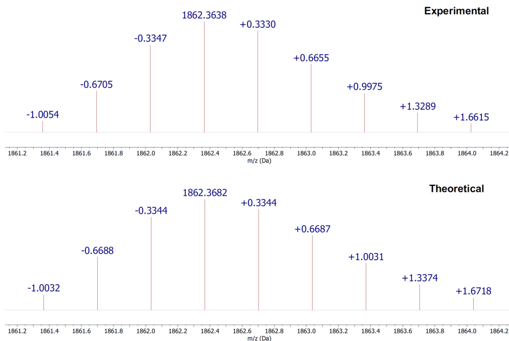
Figure S3c-3. Isotope distributions of ion \text{H16}\cdot(\text{OV}^{2+})_2\cdot\text{PF}_6^- in the 1:4 mixture of H16 and \text{OV}^{2+}\cdot(\text{PF}_6^-)_2 (upper: from ESI-QTOF spectrum; bottom: from computer simulation). The mass difference between isotope peaks is about 0.33 (1/3).
