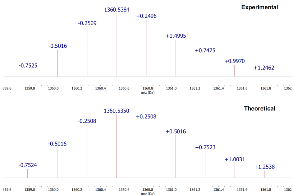
Figure S3b-2. Isotope distributions of ion \text{H16}\cdot(\text{OV}^{2+})_2 in the 1:2 mixture of H16 and \text{OV}^{2+}\cdot(\text{PF}_6^-)_2 (upper: from ESI-QTOF spectrum; bottom: from computer simulation). The mass difference between isotope peaks is about 0.25 (1/4).
