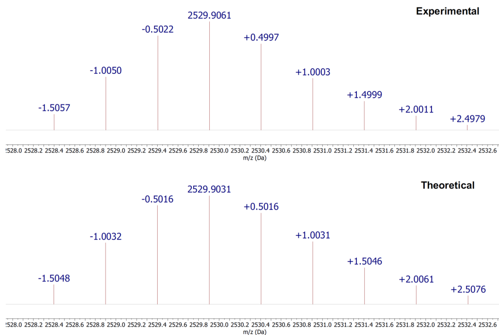
Figure S3a-2. Isotope distributions of ion \text{H16}\cdot\text{OV}^{2+} in the 1:1 mixture of \text{H16} and \text{OV}^{2+}\cdot(\text{PF}_6^-)_2 (upper: from ESI-QTOF spectrum; bottom: from computer simulation). The mass difference between isotope peaks is about 0.5 (1/2).
